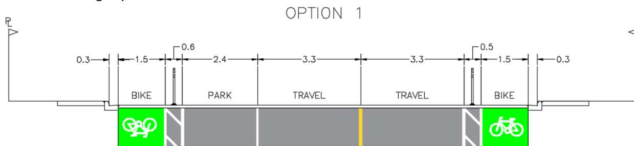
Figure 2: Option 1 - separated bike lanes on the north and south side
